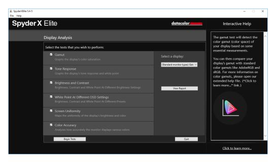
Select the tests you wish to perform and then click "Begin Tests." The software will walk you through where to place the sensor and direct you when to change the brightness on your display.
