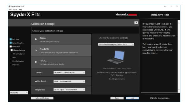
It will measure a small amount of color patches and either give you two checks or one or two X's, which mean you will need to recalibrate.
