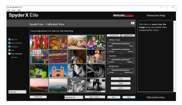
When done properly, a StudioMatch calibration will match multiple displays. If you are using multiple displays and they work with different backlight technologies and different panels, it gets complicated to match them together. That's where the SpyderTune function of SpyderX comes in.
