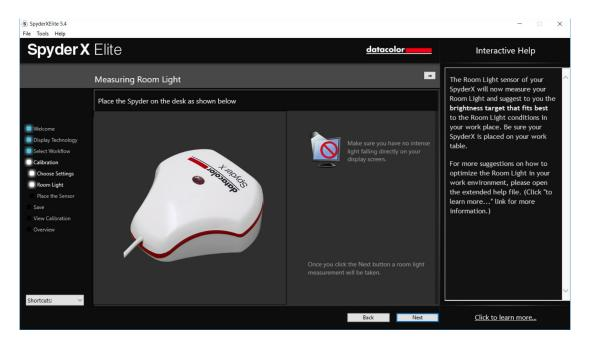
Next you will take brightness readings of the displays you are looking to match. The software will keep track of these displays and when finished, it will recommend settings based on its readings. It will give you a targeted brightness, keep track of this number if you are going to try to match monitors connected to another machine, it will also give you recommended gamma and White Point settings based on its readings.
