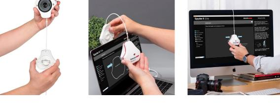
Once the unit is in place, click the next button to proceed with the calibration. A series of color patches will flash on the screen, this process takes approximately 2-3 minutes.
