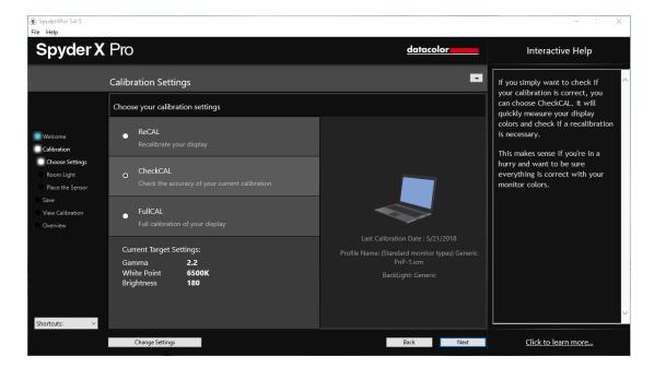
It will measure a small amount of color patches and either gives you two checks or one or two X's, which mean you will need to recalibrate.
