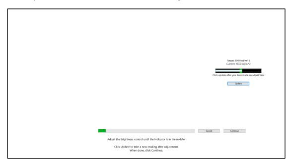
When you are within the parameters, you can press the "Continue" button. It may take a couple of times to get your brightness set properly, please try to get as close as possible to the target, though it may not fall completely within the range, that is ok, as long as you are as close as you can be.
